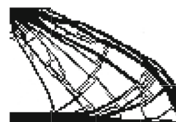
Fig. 9 Results for compliance minimization using a SIREN neural network. No density filter is applied, and all other settings are kept fixed except for the frequency parameter \omega_0 . As \omega_0 increases, high-frequency oscillations emerge in the density field, leading to checkerboard-like patterns
