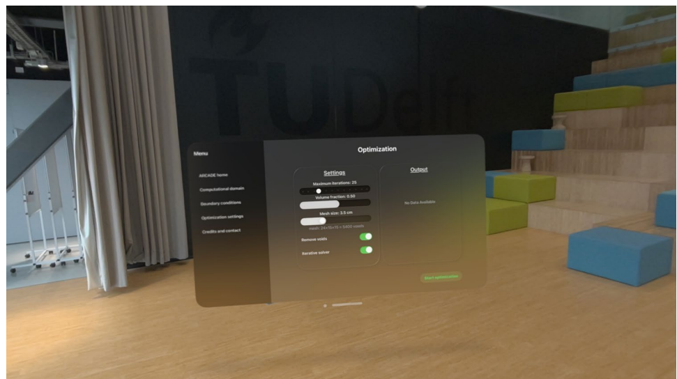
Fig. 3 Settings that define the optimization are set in the “Optimization settings” tab. These include the maximum allowed number of iterations, the target volume fraction of material within the computational design domain, and the finite element mesh size used for the discretization. The toggles allow the removal of voids during optimization and to use an iterative solver (both set to true by default)
