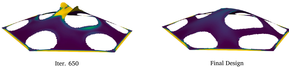
Fig. C.16. 3D rendering of the linear modal stiffnesses depicted in Fig. 10, for iteration 650 and the final design. A threshold of \bar{\rho}_i \geq 0.5 and a domain deformation corresponding to the fundamental mode shape was applied for clarity.
